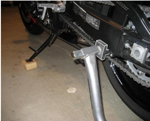
USING UNIVERSAL "L" SHAPED PADS
